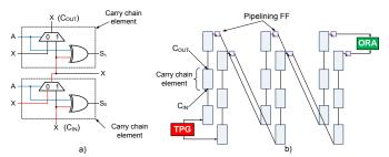
Fig. 4: Carry chain test architecture: (a) Two-stage chain under test (b) Pipelined test setup
