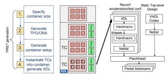
Fig. 5: XDL file generation flow for CLB TCs; Partial reconfiguration flow for test configurations
