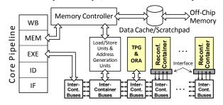
Fig. 1: System architecture with integrated test pattern generator (TPG), output response analyzer (ORA), and reconfigurable containers [8]
